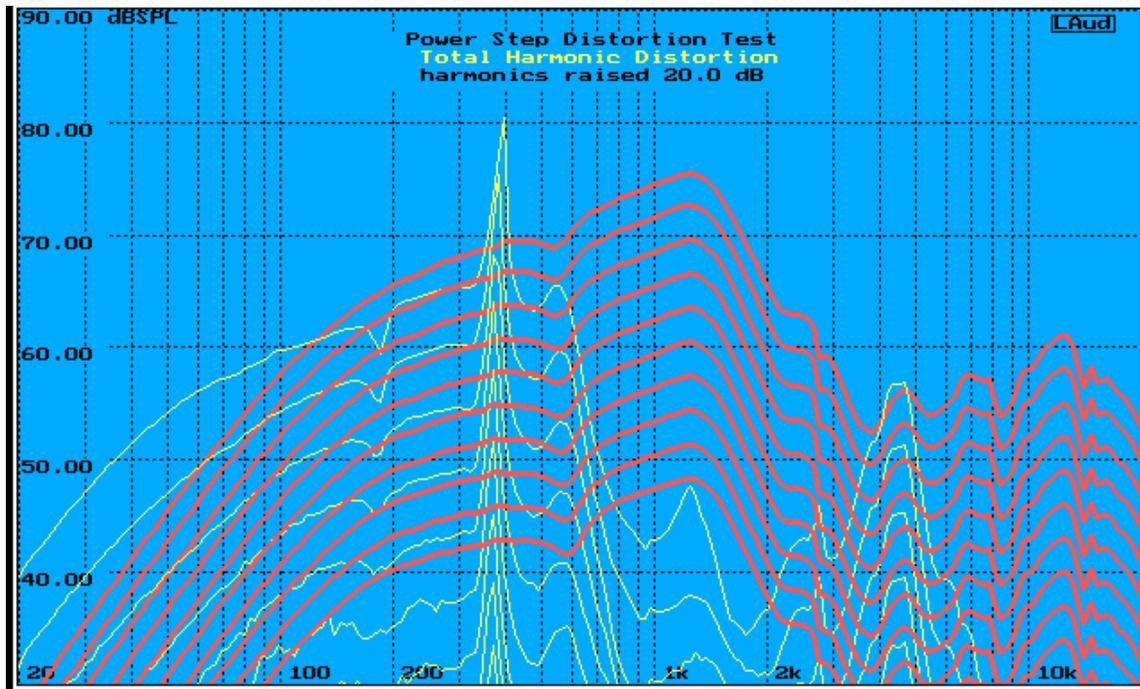
BEB prototype in ear headphones- step response mic input attenuated -40db
